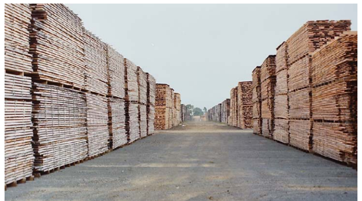
An example of good environmental controls against sapstain with no mud, timber above a layer of gravel, timber racked out and not block stacked and adequate ventilation between timber stacks.
